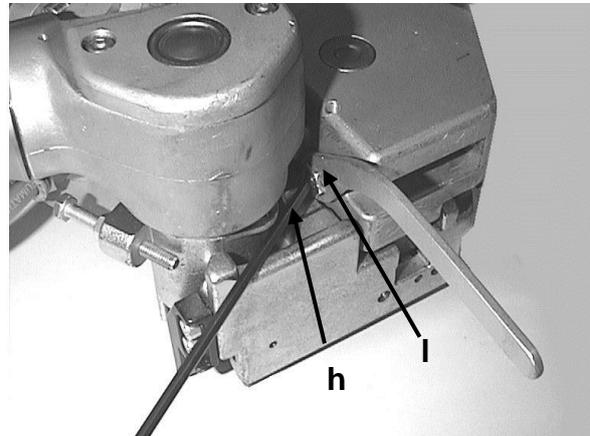
Fasten lock nut **(l)** using spanner after adjustment has been completed.
