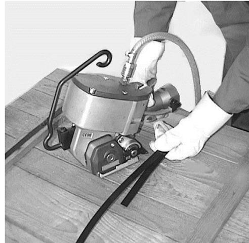
3. Hold both of the precisely overlapping straps firmly using your left hand. Using your right hand take hold of the lifting lever **(c)** and compressed air motor **(f)** and press together. Push both straps laterally along the housing wall into the tool as far as possible. A bit of the lower strap has to project out of the front of the tool. Release the lever **(c)** and motor **(f)**.
