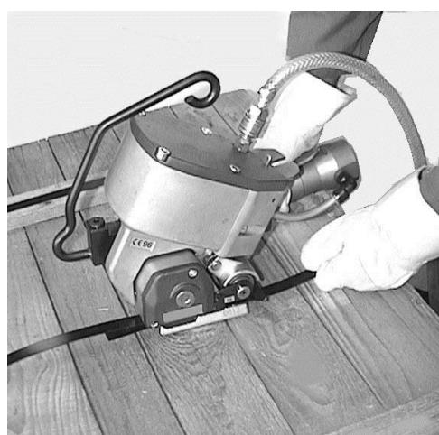
4. Use your right thumb to press the „tension strap“ key button **(a)** until it engages the notch **(g)** (the compressed air motor Stops if the notch released) For **PKE-HD** tools having built-in-free-wheeling mechanisms the “tension strap” key button **(a)** should be pressed until the desired strap tension has been achieved.
