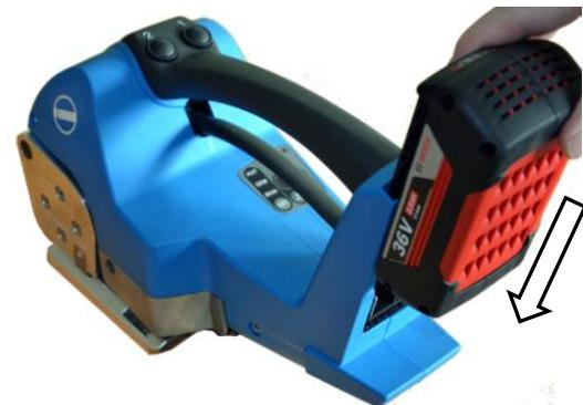
**To enable the tool please press push-button 1 for a short moment.** The LED signal lamp flashes. The TA750 is ready for operation.
