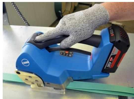
**Pull the lever 3 toward the grip and hold it. Now the strap is released. Turn the strapping tool to the right side away from the strapping while holding the lever.**
