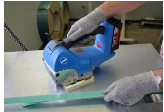
**Pull both straps to the stop along the side of the housing wall into the tool.**
