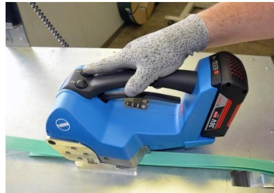
**To form a seal push push-button 2. Friction welding starts.**
