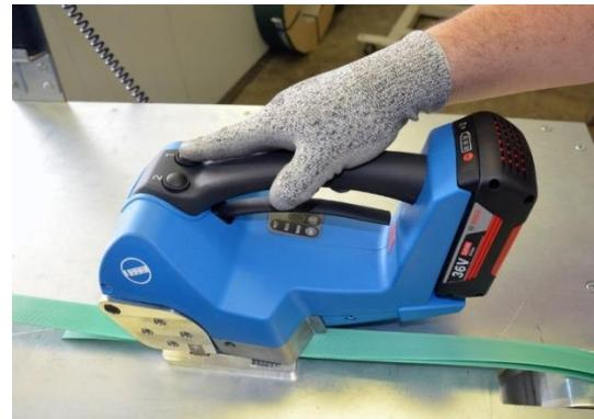
**Pull the lever 3 toward the grip and hold it. Now the strap is released. Turn the strapping tool to the right side away from the strapping while holding the lever.**
