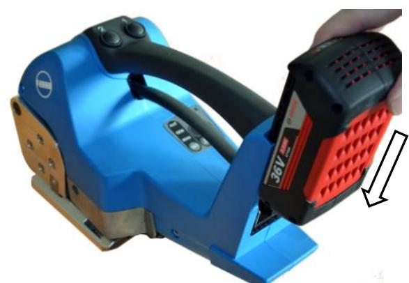
Afterwards plug the charged Li-Ion battery (130) into the slot provided till the stop is reached.
