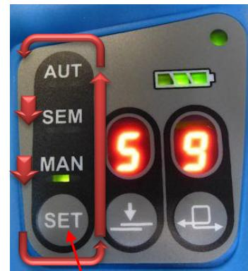
b.) Afterwards press the SET button as long as the desired operation mode starts flashing.
